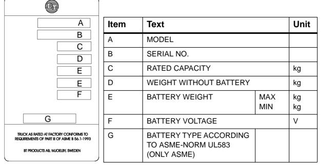
The illustration shows the identification plate for the truck in ASME-design.
