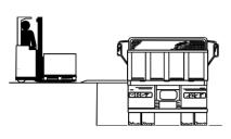
An overloaded lift can fall out of control down the lift shaft. Always check the capacity of the lift before driving in with the truck.
