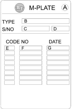
The illustration shows the modification plate which is found on the truck if it is supplied as non-standard or if it has been modified after leaving the manufacturer. The plate includes information according to the table below.
