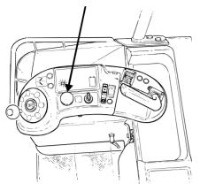
The truck is equipped with emergency switch off (see illustr.). Press in the emergency switch off to cut the power supply in the event of:
