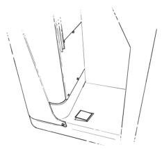
An emergency stop can be performed on the truck by removing your left foot from the foot pedal. This give full braking force without delay.
