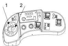
When small steering wheel adjustments are required and when driving at high speed, steer the truck with the finger-tips on the steering wheel hub (1). For low speed driving and turning the truck, rotate the wheel faster with the help of the steering wheel spinner (2).
