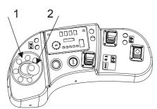
When small steering wheel adjustments are required and when driving at high speed, steer the truck with the finger-tips on the steering wheel hub (1). For low speed driving and turning the truck, rotate the wheel faster with the help of the steering wheel spinner (2).
